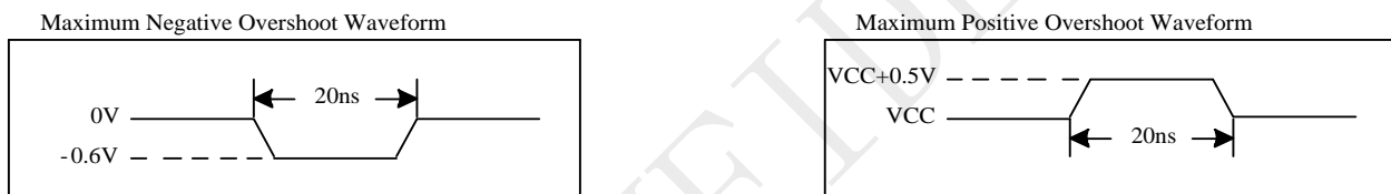
Figure 5-1 Maximum Overshoot Waveform
